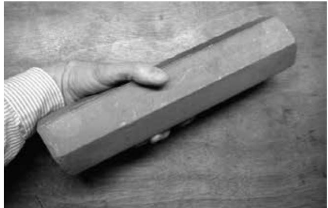
Figure 11: Anode Bar
