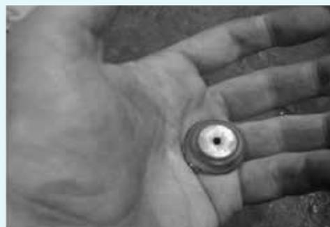
Figure 6: Orifice Plate
