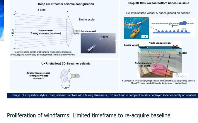
Offshore "Deep" Long streamer remain most cost effective. Hybrid streamer/OBN improves the accessibility limits Colocation
