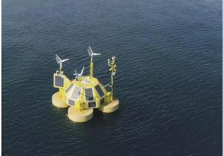
Figure 4.8: Typical Floating Lidar Buoy [15]
