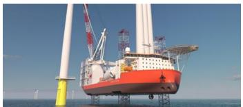
Figure 4.10: Typical Jack-up Installation Vessel
