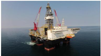
Figure 4.23: Typical Semi-Submersible Drilling Rig
