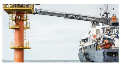
Figure 4.12: Typical Service Operation Vessel with Walk-to-Work Platform
