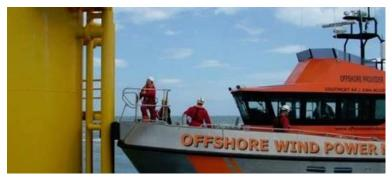
Figure 4.13: Typical Crew Transfer Vessel
