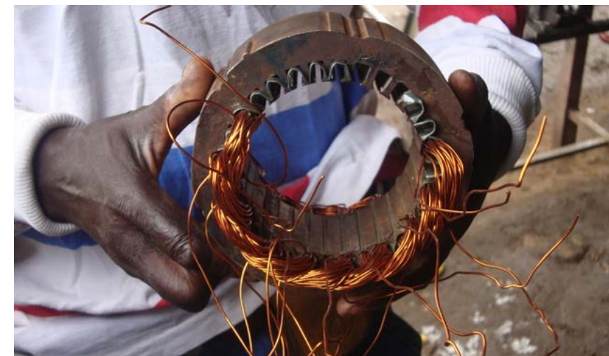
Caleb re-winding a car alternator to turn it into a home-made wind turbine.
