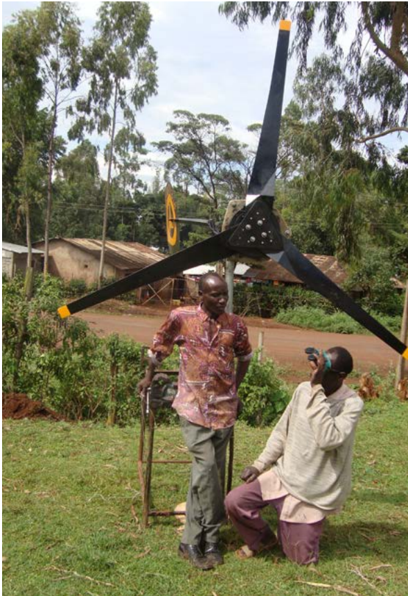
Willis, Ninja and the 700W 'Night Heron' wind turbine they built from scratch.
