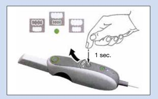
4. Hold the CS 3500 at a 90-degree angle to the occlusal surface of the preparation area. Rest the tip on the tooth surface to steady the CS 3500. Live video is displayed on the video preview screen.
