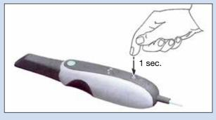
4. Let the CS 3500 warm up for approximately three minutes to enable the antifog feature on the tip.
