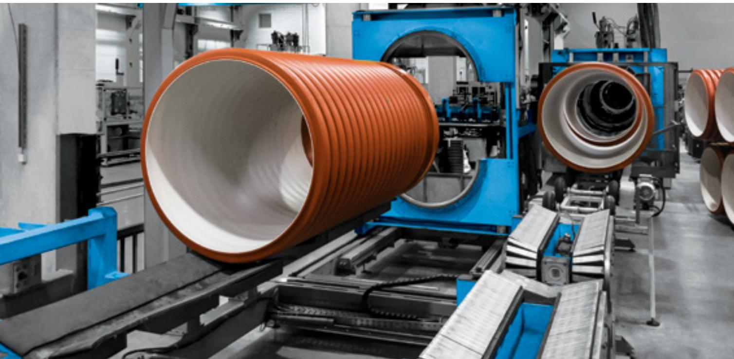
The **K2-Kan** pipes (**DN/ID** and **DN/OD**) are manufactured by co-extrusion in which two independent single-screw systems plasticize the PP granulate (of varying colours, but similar properties) which is fed to the head forming both pipes coaxially at the same time.
