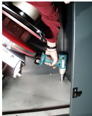
Turning out the rollers →
