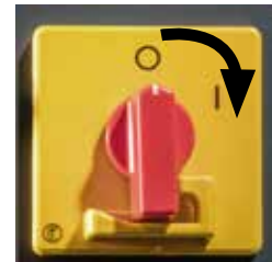
Switching on the main switch
