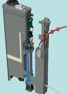
TINTA's tintONE is an intelligent one-circuit dispenser unit. Air sealed and free of stirrers it prevents the dry-out of colorants. Thanks to a significantly reduced number of moving parts in the canister, tintONE is low in maintenance and extremely service-friendly.
