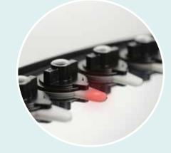
Figure 1.10: Lid monitor (LED) and software guided filling process
