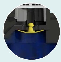
*Figure 1.8b: Closed umbrella valve during standbay and dispensing*
