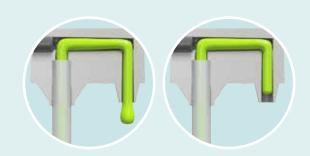
Figure 1.5: Sniffing-back the colorant into the nozzle to avoind dropping
