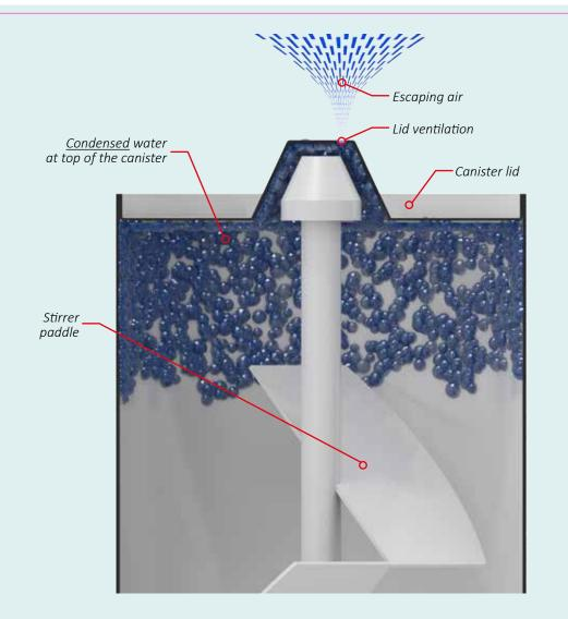
Figure 1.9: Typical free ventilation through lid of canisterns with stirrers
