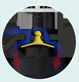
Figure 1.8a: Open umbrella valve and inflow during pump stroke for filling the piston pump
