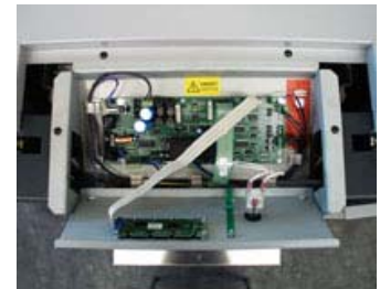
Control panel flipped down
