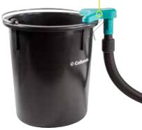
Simply clamp the dust.EX dust extraction device to the edge of the mixing bucket in combination with a vacuum cleaner. The clamping spring enables attachment to almost any mixing bucket. Switch the vacuum cleaner on for virtually dust-free working while filling or mixing. dust.EX reliably removes any escaping material.
