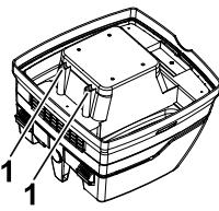
Regularly clean the water level sensors (1) and inspect for signs of damage. |
