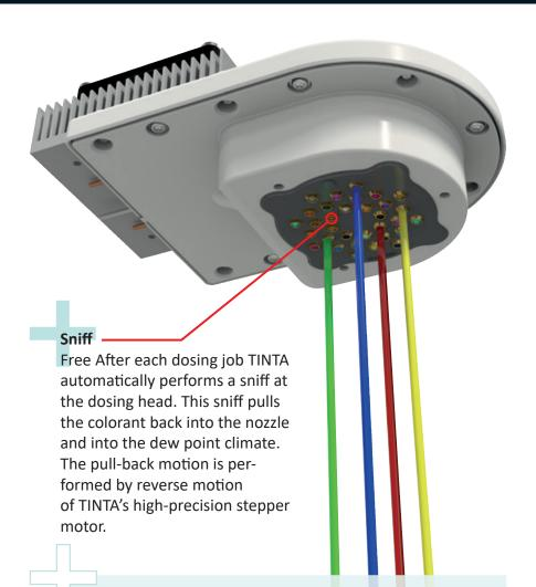
TINTA Dispensers use a proprietary and patented Collomix technology called cool**NOZ** to reduce nozzle clogging to an absolute minimum. cool**NOZ** builds upon the physical dew point principle.
