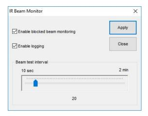
When the beam monitoring is enabled, a message box along with a shaded a vertical and/or horizontal bar will pop up to indicate the failed beams or blocked area. Touch will not function within the shaded area on the display until the failed condition is corrected.
