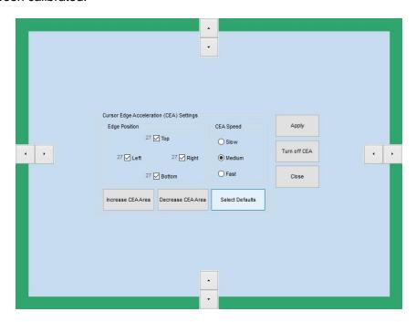
To enable CEA, click on the "Select Default" button and specify the desired parameters. The position of CEA may be manipulated for all edges at once by means of the "Increase/Decrease CEA Area" buttons, or individually by means of the arrows along each edge. Additionally, CEA for particular edges may be disabled by unchecking their respective box.
