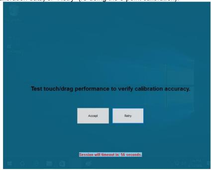
Note: Some advanced settings under "Touch Screen Properties" will not be configured until the touch screen has been calibrated.
