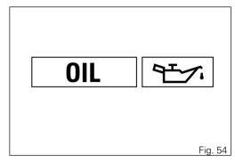
OIL SERVICE or ANNUAL SERVICE or DESMO SERVICE countdown indication After Oil Service zero indication first reset (at 1,000 km - 600 mi), the instrument panel activates the following indications in yellow for 5 seconds upon Key-ON:
