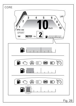
Note In case of fault or error of the fuel level sensor, no level marks will be displayed, the fuel pump symbol will be red and flashing, and the Fuel Range warning light will be on.
