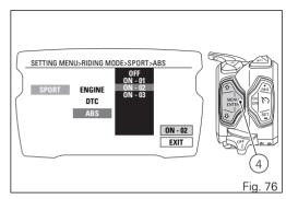
When entering the function, the currently set ABS level or status is indicated on the right (above the word EXIT) (e.g.: ON - 03, i.e. level 03). Customisation options are indicated on the central drop-down menu: levels 1 to 3 and status OFF. Press buttons (1) and (2) to highlight the levels one by one: in particular, use button (1) to highlight the following item and button (2) to highlight the previous item.
