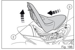
Remove the passenger seat (4) by sliding it from the motorcycle front side.
