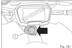
Key-On can only occur in the presence of one of the two keys (3) or (4) or using the pin code. Key-Off can also occur without any key (3) or (4). Key-Off occurs when motorcycle speed is equal to zero, by pressing button (6, Fig. 150)on the handlebar or by pressing the Hands free button (7). When speed other than zero, perform key-off by pressing the Hands free button (7).
