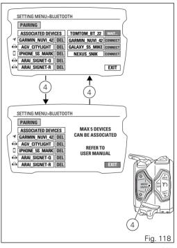
When the device to be paired has been selected, the label in correspondence of that device replaces the word "CONNECTED" with "WAIT" and it is necessary to select the type of device to be paired. The display shows four icons that represent the available types. Types of devices can be:
