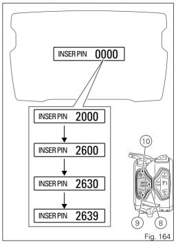
When you press function button (8) of the left-hand switch to confirm the fourth and last digit:
