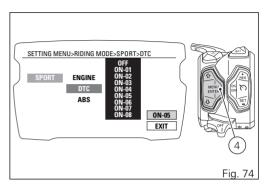
When entering the function, the currently set DTC level or status is indicated on the right (above the word EXIT) (e.g.: ON - 05, i.e. level 05). Customisation options are indicated on the central drop-down menu: levels 1 to 8 and status OFF. Once the desired new setting is highlighted, press button (4) to highlight MEMORY in orange. To save the new setting, hold button (4) for two seconds while the message MEMORY is highlighted in orange.
