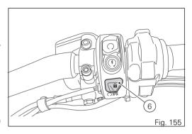
Key-On/Key-Off using the button on the Hands free lock with the active key
