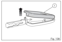
After separating the plastic shells, remove the battery protection cap (2).
