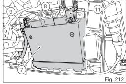
Connect the battery charger leads to the battery terminals: the red one to the positive terminal (+), the black one to the negative terminal (-).
