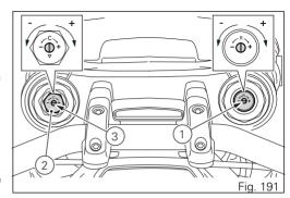
The stiffest damping setting is obtained with the adjuster turned fully clockwise to the "0" position. By turning counter clockwise starting from this position, count the clicks that will correspond to positions "1", "2" etc.
