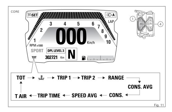
From the main screen, with TRACK layout, press button (1) on LH switch to view Menu 1 information.
