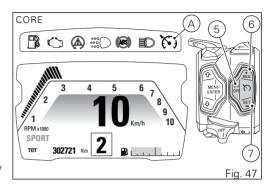
Once the system is on, it is possible to set the current speed as target speed by pressing the SET button (7). If no target speed had been previously set, it will be possible to set the current speed as target also by pressing the RES button (6) instead of button SET (7). In this case, the system saves the vehicle current speed and keeps it without having to work on the twistgrip.
