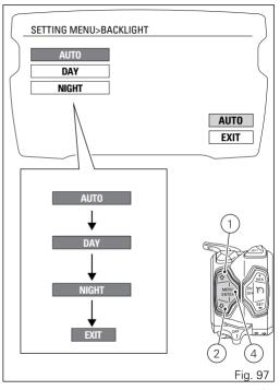
Select DAY (day mode) to permanently set display "white" background for improved readability - recommended in conditions of strong ambient light. Select NIGHT (night mode) to permanently set display black background for dimmed visibility - recommended in case of poor ambient light and/or at night.
