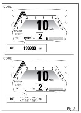
The reading is not lost in case of a power OFF (Battery OFF).
