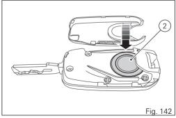
Reinstall the rear plastic shell and push slightly as shown in the figure.
