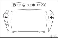
Once the "Hazard" function is activated, if vehicle is turned off (key turned to "OFF"), the function stays active for 2 hours. After 2 hours, the turn indicators switch OFF automatically in order to save battery charge.
