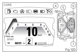
Once the system is on, it is possible to set the current speed as target speed by pressing the SET button (7). If no target speed had been previously set, it will be possible to set the current speed as target also by pressing the RES button (6) instead of button SET (7).
