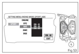
When entering the function, the currently set ABS level or status is indicated on the right (above the word EXIT) (e.g.: ON - 03, i.e. level 03).
