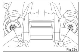
The stiffest damping setting is obtained with the adjuster turned fully clockwise to the "0" (fully closed) position.
