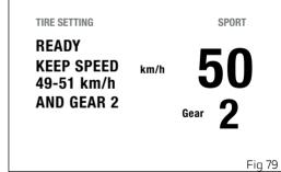
When the rider complies with the required conditions of vehicle speed and gear displayed, the instrument panel starts system calibration: all previous information will be displayed showing "IN PROGRESS" instead of "READY" (Fig 80).
