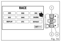
When entering the function, currently set engine power is indicated on the left (e.g.: ENGINE HIGH). Customisation options are listed on the right:
