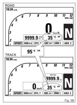
If the air temperature sensor is in fault, the instrument panel will show three flashing dashes " - -- " as air temperature value, followed by the unit of measurement, the EOBD light will turn on and the corresponding error (T AIR SENSOR) is displayed. If the instrument panel is not receiving air temperature value, a string of three steady dashes "- - -" is displayed, followed by the unit of measurement.
