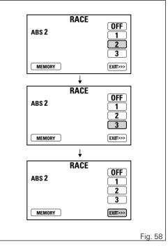
To save the new setting, hold button (4) for 3 seconds while the message MEMORY is highlighted in orange. If storage is successful, MEMORIZED will be highlighted in green for 1 second, level number or status will be refreshed (update is indicated in green) and then EXIT will be highlighted in green. To exit the menu and go back to previous page, select
