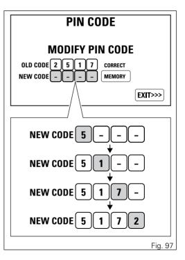
When you press button (4) to confirm the fourth and last digit, the instrument panel highlights the message MEMORY.
