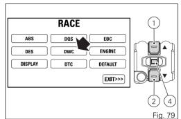
Note If DTC is set to OFF, also the DWC is automatically disabled and it will not be possible to gain access to the corresponding setup page.
