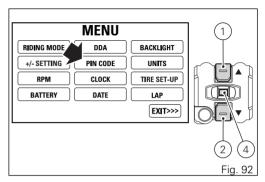
When entering the function, the display shows the message INSERT PIN CODE followed by four green dashes "- - - -".
