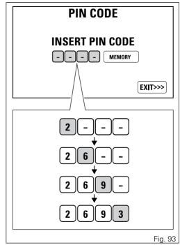
When you press button (4) to confirm the fourth and last digit, the instrument panel highlights the message MEMORY.
