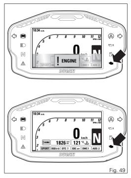
If several errors are active, the corresponding icons will be displayed one after the other, each remaining on display for 3 seconds.
