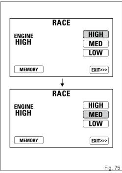
Press buttons (1) and (2) to highlight the available power options one by one: in particular, use button (1) to highlight the following item and button (2) to highlight the previous item.
