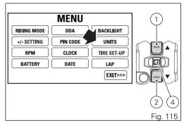
When entering the function, the display shows on the left the list of values for which units of measurements can be set:
