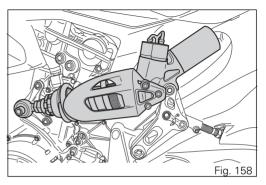
For shock absorber adjustment, follow the description on page 137. Spring preload: 12 mm.
