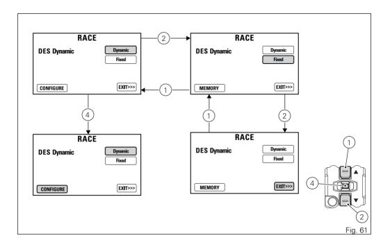
When the parameter corresponding to the nonactivated mode is highlighted, MEMORY is displayed instead of CONFIGURE: press button (4) to select MEMORY and press button (4) again for 3 seconds to activate the mode.
