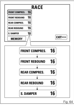
Press buttons (1) and (2) to highlight the customisable parameters one by one: in particular, use button (1) to highlight the following item and button (2) to highlight the previous item.
