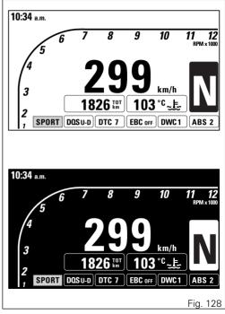
Note If power is above 16 V, backlighting is disabled, while if power is below 8 V, backlighting is turned off.
