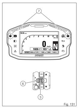
After activating the "Hazard" function, if motorcycle is switched OFF (key set to OFF), the function stays active until manually disabled by user or as long as battery voltage is (higher than or equal to) 12.2 V. When voltage drops < (below) 12.2 V the turn indicators switch OFF automatically in order to save battery charge.
