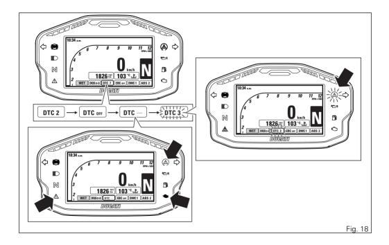
The Ducati Traction Control system (DTC) supervises the rear wheel slipping control and settings vary through eight different levels that are calibrated to offer a different tolerance level to rear wheel slipping. Each Riding Mode features a pre-set intervention level. Level 8 indicates system intervention whenever a slight slipping is detected, while level 1 is for track use and very expert riders because it is less sensitive to slipping and intervention is hence softer
