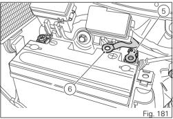
Connect the positive cable (5), previously assembled to ABS cable (6), to battery positive terminal, and negative cable (7) to battery negative terminal, by starting the other screw (4).
