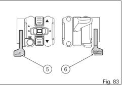
When entering the function, the currently set function associated with the UP + and DOWN buttons is indicated on the left (e.g.: DTC). Customisation options are listed on the right: DTC, DWC or EBC.
