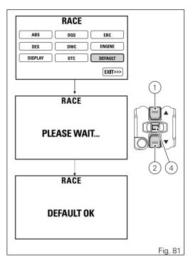
It will take 3 seconds to restore parameters, during which PLEASE WAIT... will appear on the display. Once procedure is completed, DEFAULT OK will appear for 2 seconds to confirm that default parameters have been restored.
