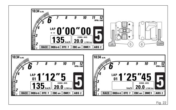
Any time rider pushes the UP + button (5) the level of the associated function is increased by one until the maximum level available is reached (DTC 8, DWC 8, EBC 3); if the button is pressed for a few seconds, the increase continues until the button is released or until the maximum level available is reached.
