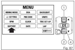
If the battery voltage error is present, the instrument panel will show three flashing dashes "---" as voltage value, followed by the unit of measurement, the Generic Error light will turn on and the corresponding error (BATTERY) is displayed.
