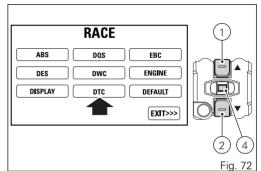
When entering the function, the currently set DTC level or status is indicated on the left (e.g.: DTC 3). Customisation options are indicated on the right: levels 1 to 8 and status OFF.
