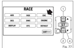
When entering the function, the currently set EBC level or status is indicated on the left (e.g.: EBC 1). Customisation options are indicated on the right: levels 1 to 3 and status OFF. Press buttons (1) and (2) to highlight the levels one by one: in particular, use button (1) to highlight the following item and button (2) to highlight the previous item. Once the desired level is highlighted, press CONFIRM MENU button (4) to highlight MEMORY.
