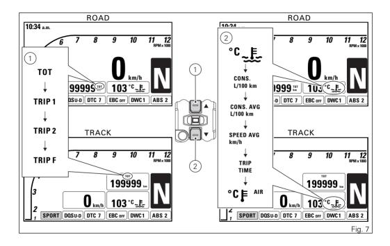
When the Standard Screen is displayed, hold the button (2) for 3 seconds, when actual motorcycle speed is <= (lower than or equal to) 20 km/h, to enter the Setting MENU, where you can set any function.
