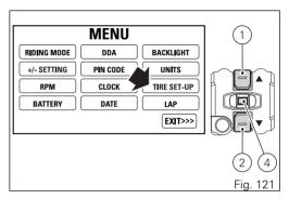
Press buttons (1) and (2) to select START or DEFAULT: the latter can be selected only if the motorcycle is currently not set to the factory default configuration.
