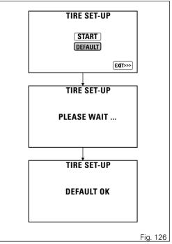
While, if the procedure for restoring the default settings is not successful, ABORTED will be displayed for 2 seconds and then the instrument panel will automatically display the main screen of the TIRE SET-UP menu with highlighted EXIT item.
