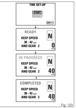
If it is not possible to start the procedure when the START is confirmed, after a few seconds the instrument panel will automatically highlight the option EXIT.
