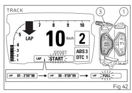
If the LAP function is not selected from the menu, the instrument panel will go back to the functions present before the FLASH button (3) was pressed. It is possible to scroll the other menu functions at any time.
