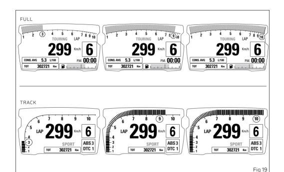
When the threshold before the rpm limiter is reached, the corresponding warning lights will turn on.
