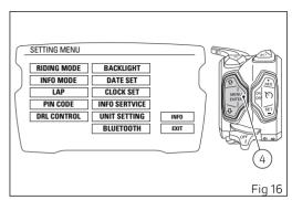
If the key is not acknowledged upon Key-On and once the check routine is over, if the PIN CODE function is active the instrument panel shows a screen where it is possible to enter the release PIN CODE. Use button (1) and button (2) to enter the code digit and confirm by pressing button (4).
