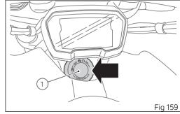
Key-On can only occur in the presence of one of the two keys (3) or (4) or using the pin code. Key-Off can also occur without any key (3) or (4). Key-Off occurs when the speed of the motorcycle is equal to zero, by pressing button (6, Fig 158) on the handlebar or by pressing the Hands free button (1). When speed is not equal to zero, perform key-off by pressing the Hands free button (1).
