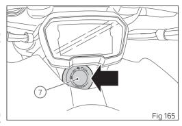
Key-On/Key-Off using the button on the handlebar with the passive key.
