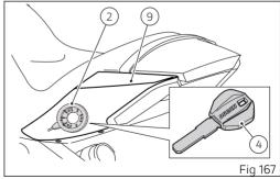
Key-On/Key-Off using the button on the Hands free lock with the passive key
