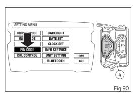
When entering the function, the display shows the message INSERT NEW PIN CODE followed by the first digit in green and three dashes "0 - - -". Entering the code:
