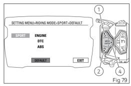
It will take three seconds to restore parameters, during which the display will show "WAIT...". Once procedure is completed, "OK" will appear for two seconds to confirm that default parameters have been restored and the message EXIT will be highlighted.
