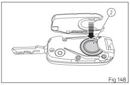
Reinstall the rear plastic shell and push slightly as shown in the figure.
