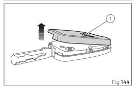
After separating the plastic shells, remove the battery protection cap (2). Remove battery (3) and install a new one.
