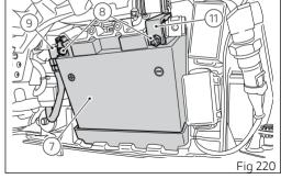
Connect the battery charger leads to the battery terminals: the red one to the positive terminal (+), the black one to the negative terminal (-).
