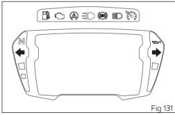
Once the "Hazard" function is activated, if vehicle is turned off (key turned to "OFF"), the function stays active for 2 hours. After 2 hours, the turn indicators switch OFF automatically in order to save battery charge.
