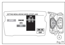
When entering the function, the currently set ABS level or status is indicated on the right (above the word EXIT) (e.a.: ON - 03. i.e. level 03). Customisation options are indicated on the central drop-down menu: levels 1 to 3 and status OFF. Press buttons (1) and (2) to highlight the levels one by one: in particular, use button (1) to highlight the following item and button (2) to highlight the
