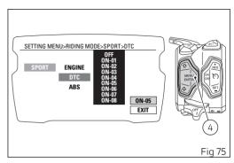
When entering the function, the currently set DTC level or status is indicated on the right (above the word EXIT) (e.g.: ON - 05, i.e. level 05).
