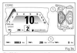
The TRIP1 counter is automatically reset in case the system unit of measurement is changed manually or after a Battery-OFF: the counter will then start back from zero, considering the new units of measurement.
