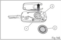
Install the battery in place, paying attention to respect polarity: positive pole (+) must be facing up.
