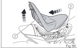
Remove the passenger seat (4) by sliding it from the motorcycle front side.
