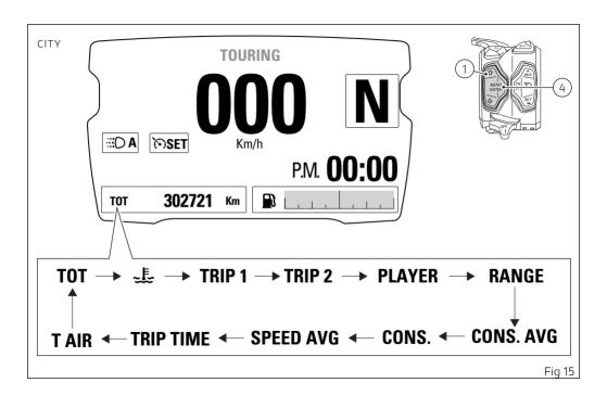
For the FULL display mode, the instrument panel stores Menu 1 and Menu 2 settings in use upon KEY-OFF. On the following KEY-ON, previously stored Menu 1 e Menu 2 pages are displayed.
