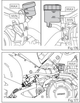
Attention Brake and clutch fluid can damage paintwork and plastic parts, so avoid contact. Hydraulic fluid is corrosive; it may cause damage and
