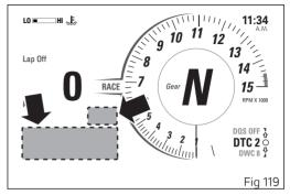
OIL SERVICE zero warning The first service warning is the OIL SERVICE zero and is triggered as soon as the odometer reaches the first 1,000 km (600 mi). Warning is displayed until reset by the Ducati authorised service centre, during maintenance.
