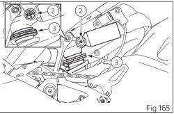
compression (2): 0.5 turns from fully closed; spring preload: 18 mm (0.71 in) from fully uncompressed spring.
