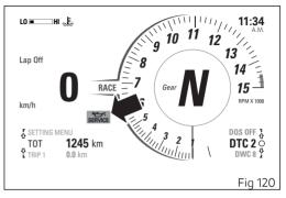
OIL SERVICE countdown, ANNUAL SERVICE countdown, DESMO SERVICE countdown When the set service thresholds are close, the instrument panel activates the following yellow warnings for 5 seconds upon every Key-ON:
