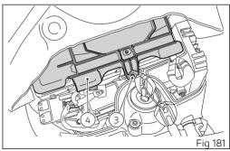
Slide out the battery (5) from its housing and, always starting from the negative terminal (-), loosen the screws (6a) and (6b). Remove the ABS positive cable (7) and positive cable (8) from the positive terminal and the two negative cables (9) from the negative terminal.
