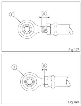
Rear brake pedal Loosen lock nut (4).
