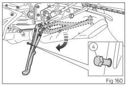
To move the side stand to its rest position (horizontal position), lean the motorcycle to the right while lifting the thrust arm (1) with your foot. To ensure trouble-free operation of the side stand joint, thoroughly clean it and then use SHELL Alvania R3 grease to lubricate all friction points.
