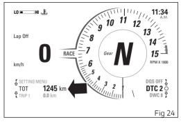
The UP 1 and DOWN 2 arrows - corresponding to the navigation buttons - appear on the LH side of the menu indicating the possibility to scroll through
