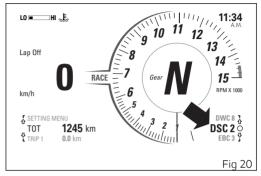
The DSC system works on 2 different levels, each calibrated to offer a different intervention on the side slipping of the tyre in combination with a specific DTC level.
