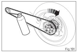
Apply the lubricant jet (1) inside the chain between the inner and outer links, in point (2) immediately before the engagement point on the sprocket.
