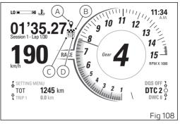
The coordinates are deleted automatically when the instrument panel detects that the motorcycles moves by more than 15 km away from the memorised coordinates.
