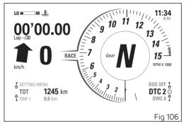
LAP BASIC with GPS module If there is a GPS module on the motorcycle, the timer start and stop is managed automatically by the instrument panel after activating the LAP function. The display shows GPS (A) symbol further to timer and lap number.
