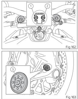
compression: Max – 7 turns (from fully closed); rebound: Max - 5.5 turns (from fully closed); spring preload: 7 turns (from fully open).
