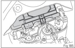
Once the tank cover (2) is positioned, tighten the four screws (1), complete with the relevant lower washers.
