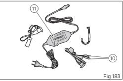
Attention Before activating the battery charger, connect it to the battery always starting with the red positive terminal (+) first.
