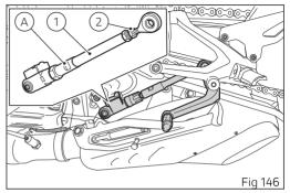
Once the adjustment is completed, check the correct value (B) of uniball travel (3). The uniball (3) travel value (B) must be between 0 mm (0 in) (uniball completely screwed in) and 6 mm (0.24 in).
