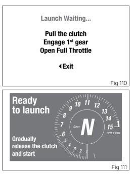
The Ducati Power Launch (DPL) helps the rider in the delicate sport starting phase from a standstill to control the power delivered by the vehicle.
