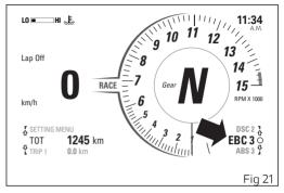
System is particularly sensitive at high rpm and sensitivity gradually decreases as soon as engine rpm decrease.
