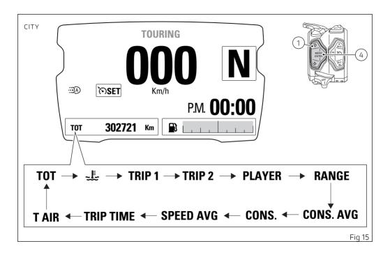
For the FULL display mode, the instrument panel stores Menu 1 and Menu 2 settings in use upon KEY-OFF. Upon the following KEY-ON, the previously stored Menu 1 and Menu 2 screens are displayed. In case of sudden and unexpected power off, the instrument panel displays the Menu 1 and Menu 2 default settings upon the following KEY-ON:
