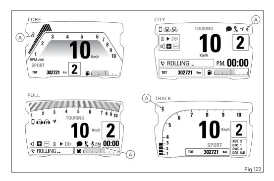
If Bluetooth is active, apart from the Bluetooth icon, also connected device indication is displayed, such as smartphone, rider and passenger helmet earphones, Ducati GPS navigator.
