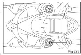
closed) position. By turning counter clockwise starting from this position, count the clicks that will correspond to positions "1", "2" etc.
