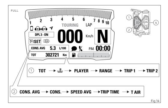
From the main screen, with CITY layout, press button (1) on LH switch to view Menu 1 information.
