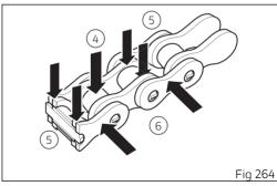
After lubrication, wait 10-15 minutes to allow the lubricant to act on the internal and external surfaces of the chain and then remove the excess lubricant with a clean cloth.
