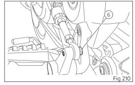
Once the adjustment is completed, check the correct value (B) of uniball travel (3).
