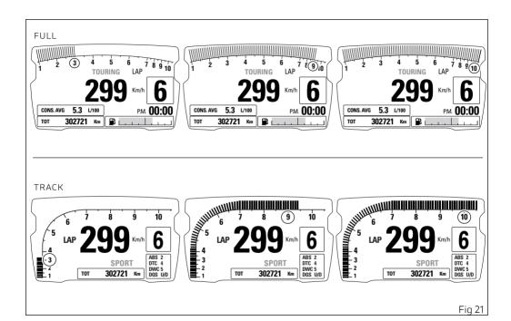
When the threshold before the rpm limiter is reached, the corresponding warning lights will turn on.
