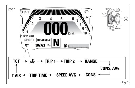
From the main screen of the TRACK mode, pressing button (1) on the left-hand switch allows displaying Menu 1 information.
