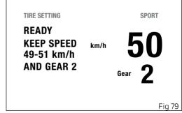
When the rider complies with the required conditions of vehicle speed and gear displayed, the instrument panel starts system calibration: all previous information will be displayed showing "IN PROGRESS" instead of "READY" (Fig 80).
