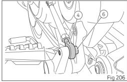
Once the adjustment is completed, check the correct value (B) of uniball travel (4).
