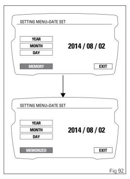
If date is not correct, the instrument panel will display "WRONG DATE" flashing for three seconds and then will automatically highlight EXIT, while date is indicated as "---- / -- " steady. It is still possible to set a new date.
