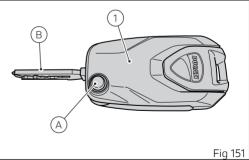
The key has a RESET button (3) of the microprocessor managing the electronic parts: if a key-on is not possible because the key is not acknowledged by the Hands Free system in active and/or passive mode, press RESET button to reenable the correct operation of the key.
