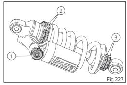
spring preload: 19±5 mm (0.75± 0.2 in) from fully uncompressed spring.
