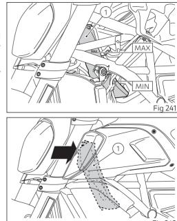
Unscrew the filler plug (2) of the expansion reservoir, on the motorcycle's right side, and add ENI Agip Permanent Spezial antifreeze (do not dilute, use pure), until reaching the MAX level. Screw plug (2).
