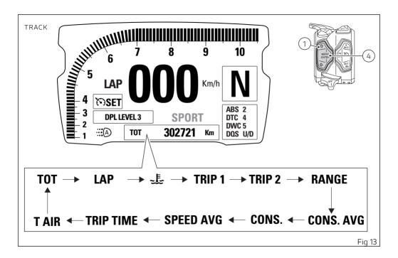
From the main screen of the FULL mode, pressing button (1) on the left-hand switch allows displaying Menu 1 information.
