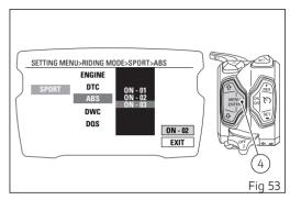
When entering the function, the currently set ABS level or status is indicated on the right (above the word EXIT) (e.g.: ON - 03, i.e. level 03).
