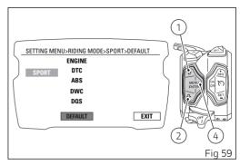
It will take three seconds to restore parameters, during which the display will show "WAIT...". Once procedure is completed, "OK" will appear for two seconds to confirm that default parameters have been restored and the message EXIT will be highlighted.
