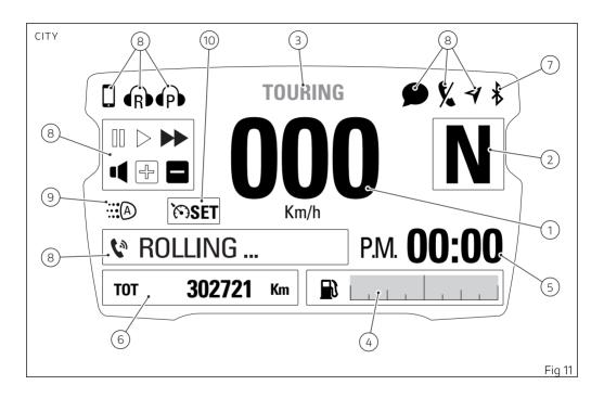
From the main screen of the CORE mode, pressing button (1) on the left-hand switch allows displaying Menu 1 information.
