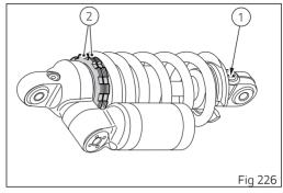
Calibration of RIDING WITH PASSENGER AND AT FULL LOAD:
