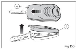
Press RESET button (3) until you hear it click. Reinstall the rear plastic cover (4) and slightly push it backward as shown in the figure. Make sure it is well closed.
