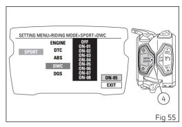
When entering the function, the currently set DWC level or status is indicated on the right (above the word EXIT) (e.g.: ON - 05, i.e. level 05). Customisation options are indicated on the central drop-down menu: levels 1 to 8 and status OFF.
