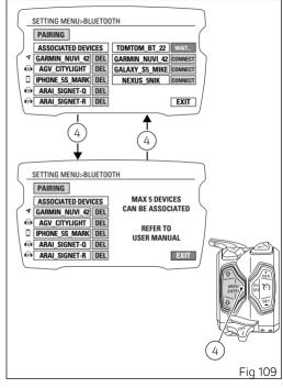
When the device to be paired has been selected, the label in correspondence of that device replaces the word "CONNECTED" with "WAIT" and it is necessary to select the type of device to be paired. The display shows four icons that represent the available types. Types of devices can be:
