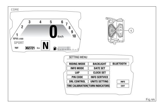
Press buttons (1) and (2) to highlight the customisable parameters one by one: in particular, use button (2) to highlight the following item and button (1) to highlight the previous item.
