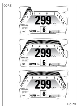
CORE layout indicates rpm in a different way compared to TRACK and FULL layouts.
