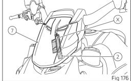
Recovery mode for Key-On with passive key and/or active key with flat battery.
