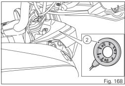
Key-On/Key-Off using the button on the Hands free lock with the passive key
