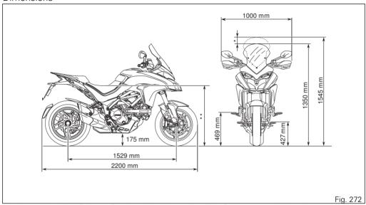
\* 1435 mm (headlight fairing at first detent), 1500 mm (headlight fairing at second detent).
