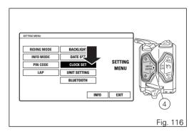
When entering the function, available settings are indicated on the left: HOUR, MINUTE, AM / PM, while set time is indicated on the right (e.g.: 10 : 30 a.m.).
