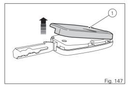
After separating the plastic shells, remove the battery protection cap (2).
