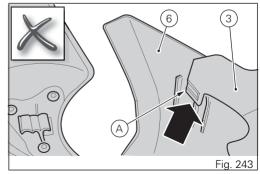
Moreover, make sure that semi-mudguard profiles are aligned as shown in the figure.
