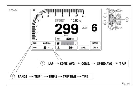
From the main screen, with FULL layout, press button (1) on LH switch to view Menu 1 information.
