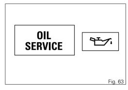
OIL SERVICE or SERVICE DATE or DESMO SERVICE countdown indication After OIL SERVICE zero indication first reset (at 1,000 km - 600 mi), the instrument panel activates the following indications in yellow for 5 seconds upon Key-ON:
