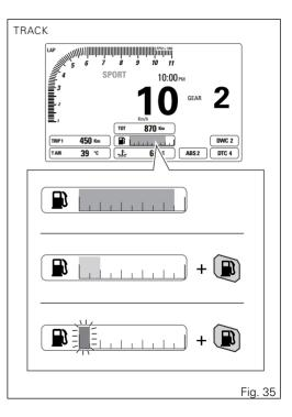
Note In case of fault or error of the fuel level sensor, no level marks will be displayed, the fuel pump symbol will be red and flashing, and the Generic Error warning light will be on.
