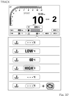
If the coolant temperature sensor is in fault, a string of flashing dashes "---" is displayed with the set unit of measurement and the MIL light turns on. If the instrument panel is not receiving coolant temperature value, a string of steady dashes "---" is displayed, followed by the unit of measurement.
