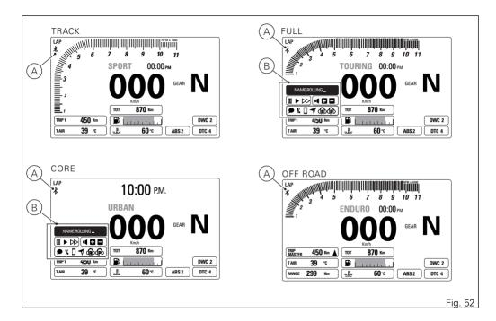
If Bluetooth is active, apart from the Bluetooth icon, also connected device indication is displayed, such as smartphone, rider and passenger helmet earphones, Ducati GPS navigator.
