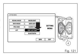
When entering the function, the display shows on the left the list of values for which units of measurements can be set:
