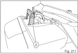
Duly engage pannier in place, making sure to properly engage hooks.
