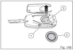
Install the battery in place, paying attention to respect polarity: positive pole (+) must be facing up.
