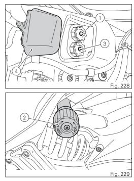
It is possible to work on adjusters (1, Fig. 228) and (3. Fig. 228) through the opening on the battery support. Manually turning the adjusters (1, Fig. 228) and (3, Fig. 228) clockwise gives harder damping, turning anticlockwise gives softer damping. Turn knob (2, Fig. 229) clockwise to increase the spring preload, or counter clockwise to decrease it.
