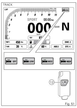
Level selection with Heated Handgrips "off": Even if heated handgrips are turned off, it is still possible to set them to LOW, MED or HIGH level, but the icon will have a white background (in DAY backlighting option of the instrument panel) or BLACK (in NIGHT backlighting option of the instrument panel).
