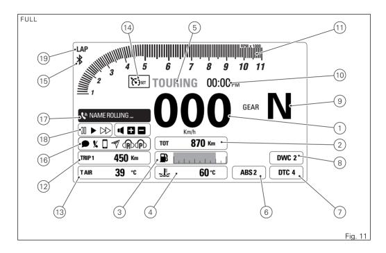
Data displayed on the main screen for CORE layout 18) LAP indication (only if active). are as follows:
