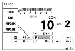
When TRIP1 is reset, the value is reset and the first value available is displayed 10 seconds after the reset.
