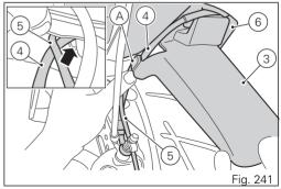
Fit the tabs (A) of front semi-mudguard kit (3) in the front mudguard (6) seat: the tabs must be inserted in the seat as shown in the figure.
