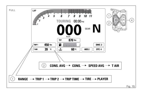
From the main screen, with CORE layout, press button (1) on LH switch to view Menu 1 information.
