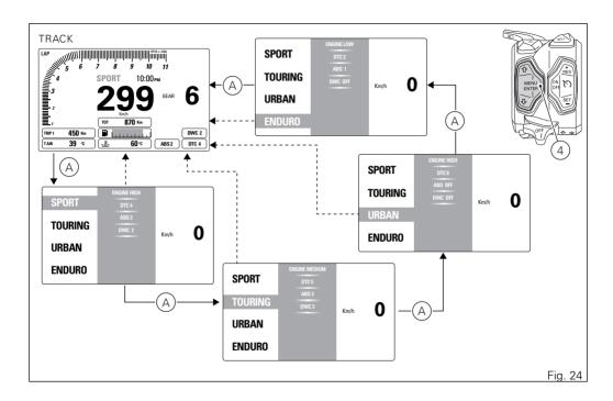
Once the desired riding mode (A, Fig. 25) is highlighted, confirm the selection by holding down the CONFIRM MENU button (4) for 2 seconds: the new riding mode selection is stored and the standard screen (C, Fig. 25) is displayed for the selected riding mode.
