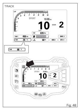
Note When the motorcycle is stopped, the engine heat could influence the displayed temperature.
