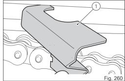
To measure the proper chain tensioning, it is necessary to check the correspondence of the chain pin axis (black line in (Fig. 261)), within the distance identified with the cutout on chain tension gauge (interval indicated by the arrows in (Fig. 261)). If chain pins are higher or lower than this interval (Fig. 262), it is necessary to tension the chain page 343.
