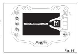
Warning reading "Steering locked" (upon Key-Off)
