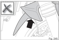
Fit the screws (2) previously removed and tighten them to a torque of 3.5 Nm  $\pm$  10%.
