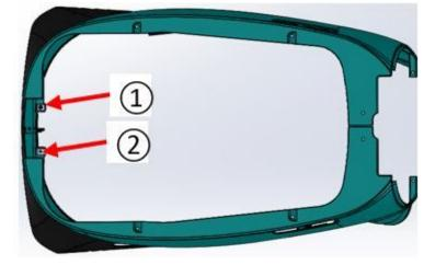
For removing each side panel, also remove the two cross-head screws.
