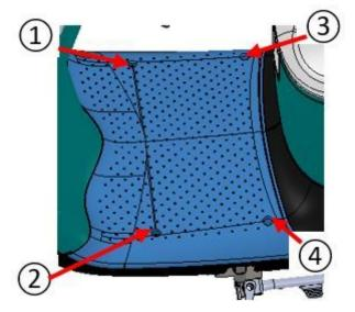
Lift up the front of the footrest panel and slide the panel towards the front by two centimeters.
