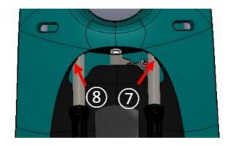
Be careful when taking off the front outer panel and detach all of the light connectors.
