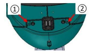
Next remove the two cross-headed screws slightly on the inside of the scooter. These screws connect to the rear side panels.
