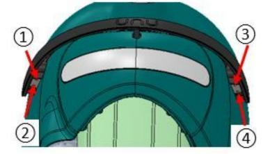
With the screws removed, stretch the ends of the handhold away from the bodykit and pull the handhold towards the rear to remove it. If you can't find the right angle for taking off the handhold, look at the angle at which the middle part of the handhold enters the bodykit. It is only slotted in and does not need to be unscrewed anywhere.
