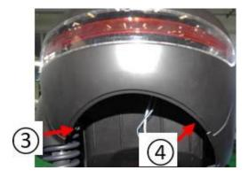
Careful when removing the rear light panel from the scooter. Make sure to unplug the connector of the rear light.
