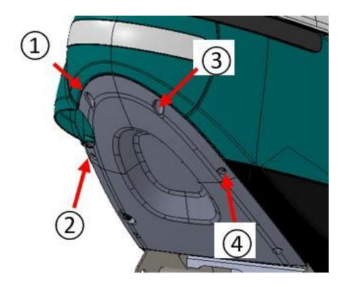
Next, let the rear panel come down a few centimeters. Careful, before removing the panel, unplug the connector of the rear charging port.
