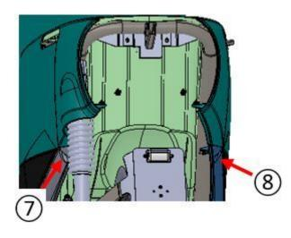
To remove the rear panel assembly, close the seat, bend the rear ends of the assembly to the side for about 20cm and slide the entire assembly forward.
