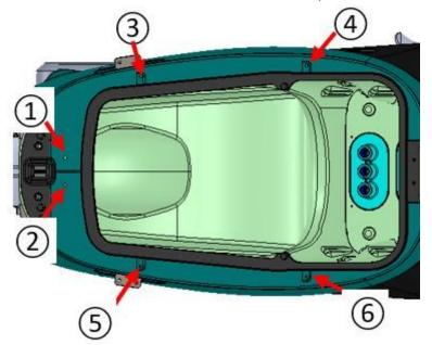
Next remove the two cross-head screws attaching the rear panels to the bottom sides.
