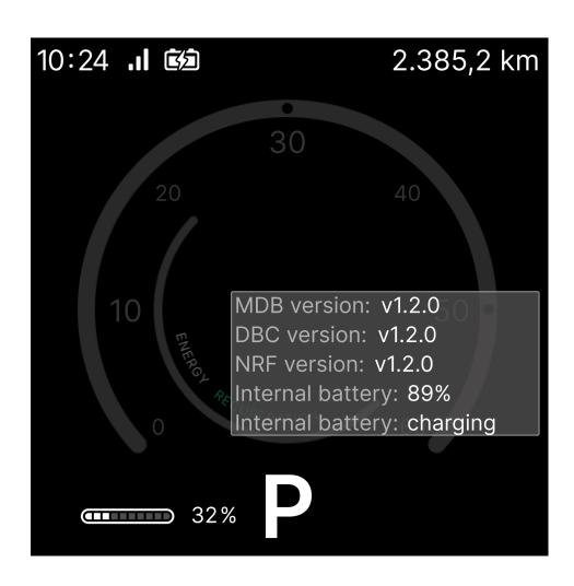
The internal battery will start recharging as soon as you reinsert a main battery and close the seat box.
