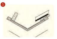
At hips, use a hip tile as a guide to find the correct position of the Rapid Roof Putty. The back of the strip must be positioned 3.5cm behind the front edge of the hip tile. Ensure all hip tiles are secured to the timber hip batten using 100 x 4mm woodscrews.
