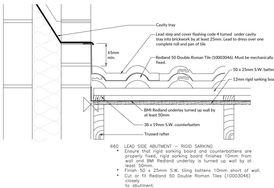
\* Ensure that code 4 lead step and cover flashing is dressed closely over one complete roll and pan of tile, turned up wall by at least 65mm, and turned under cavity tray into brickwork by at least 25mm.
