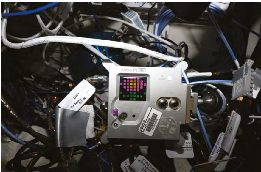
■ Mission Zero entries running on an Astro Pi on board the ISS
