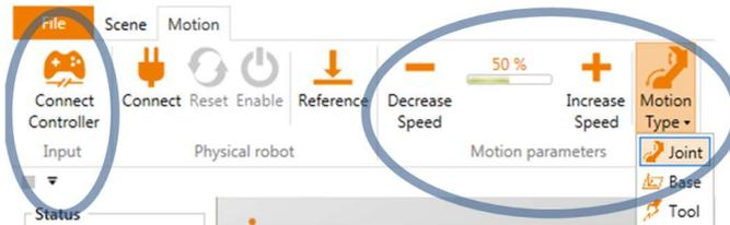
Figure 7.6 Control panel for moving the Robot (marked in blue).
