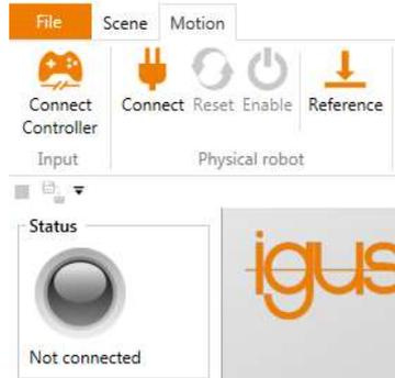
Figure 7.3 Icons for connecting to the hardware, resetting errors and enabling the motors; referencing icon; and "Status" indicator.
