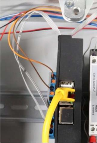
The 2 lead ribbon cable of the Embedded Computer is the RS232 connection for the Operating Panel. One lead is marked black (lead 1).
