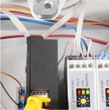
The 3 leaved ribbon cable of the Embedded Computer is the CAN connection. It has one lead marked in black (lead 1, GND). Leads 2 and 3 are CAN-L and CAN-H respectively.
