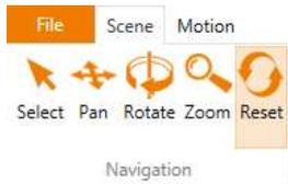
The function of the left/middle mouse button can be changed in the "Scene" tab under "Navigation", with movement options: "Select", "Pan", "Rotate", "Zoom" and "Reset".
