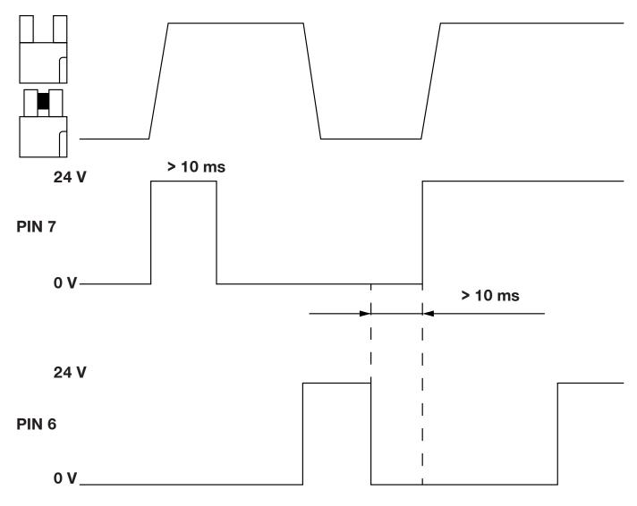
A movement in the desired direction occurs when the corresponding signal is at a high level. After a high level is detected, the gripper movement occurs until the gripping process ends.
