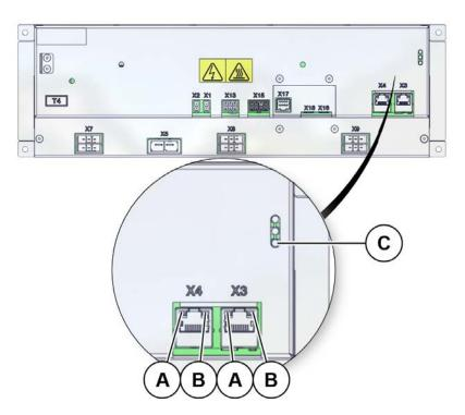
The illustration below shows the indication LEDs on the drive unit.
