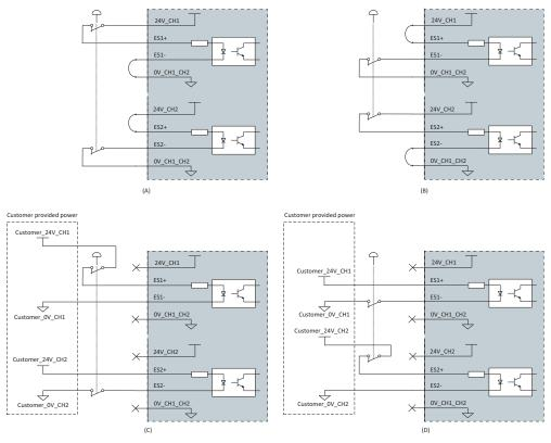
figures for the best safety performance. When the 24 V power is provided by customer instead of  $24V_CH1/2$ , it shall be within the tolerance of 24V - 5%/+5%.
