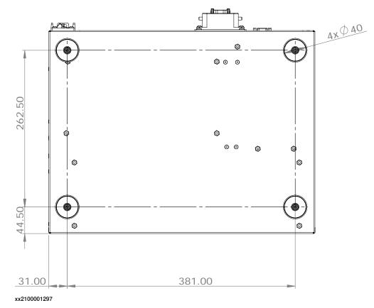
• The feet should only be used for positioning, not for mounting or fastening.
