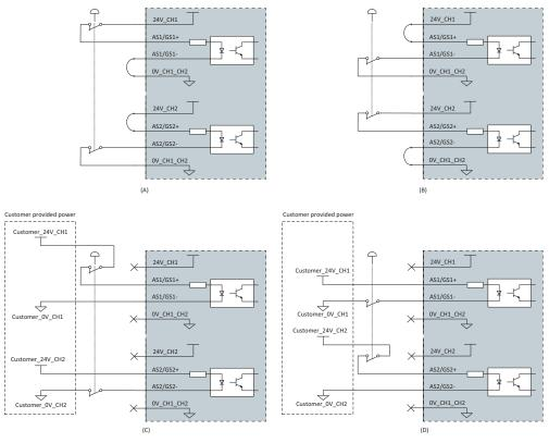
for the best safety performance. When the 24 V power is provided by customer instead of  $24V_CH1/2$ , it shall be within the tolerance of 24V - 5%/+5%.
