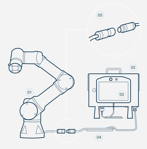
Every e-Series purchase includes a 6 m standard cable and a base flange connector that enables through-side and through-hole mounting for your robot.
