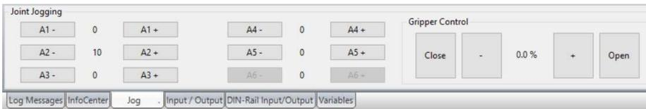
Figure 5: The buttons for joint movements. In the card safe mode, the keys change to X, Y, Z, A, B, C.
