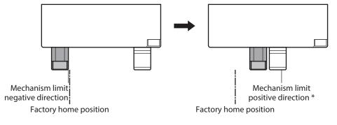
\* The mechanism limit on the positive side is set outside the moving range.
