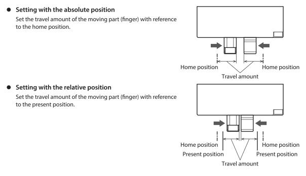
Note The operation data and parameters of the **EH** Series are set for one side of the moving parts (fingers). Setting to one side of the moving parts will also move the other side under the same conditions.
