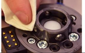
Apply a small amount of grease (Molykote BR2Plus) on the locking balls.
