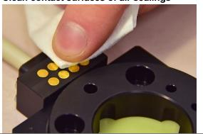
Wipe the contact surfaces of the air sealings clean with a lint free cloth.
