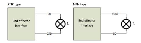
Figure 27. End effector output interface
