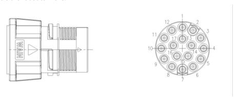
Figure 15. Handheld emergency stop and enabling device interface
