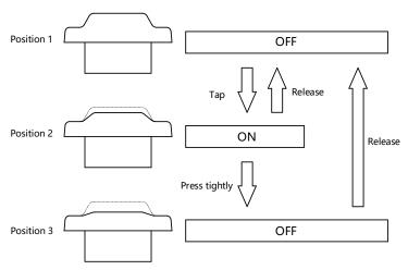
Figure 2. Positions of the enabling switch
