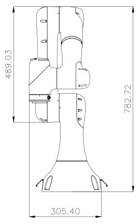
Figure 9. Reference transportation dimensions of the robot
