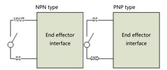
Figure 28. End effector input interface
