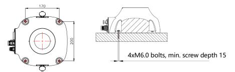
Figure 10. Reference bracket fixing method
