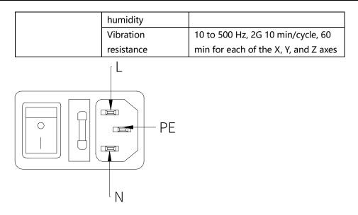
Figure 30. Power input interface
