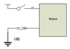
Figure 17. PNP input wiring diagram
