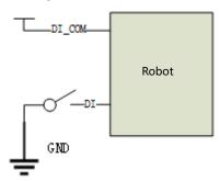
Figure 18. NPN input wiring diagram
