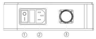
Figure 29. Power adapter interface
