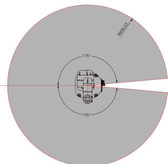
Figure 6. The working space of xMate SR4
