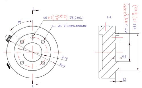
Figure 11. Tool flange installation
