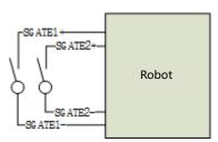
Figure 21. External emergency stop interface
