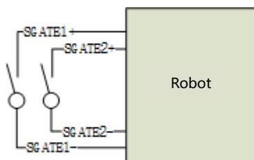
Figure 23. External emergency stop interface
