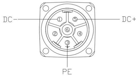
Figure 16. Power supply interface (side view for cables)
