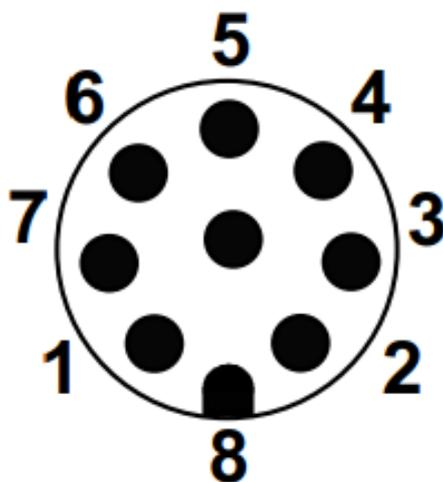
Figure 28. The end effector round connector interface
