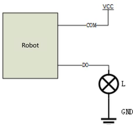
Figure 22. PNP output wiring diagram
