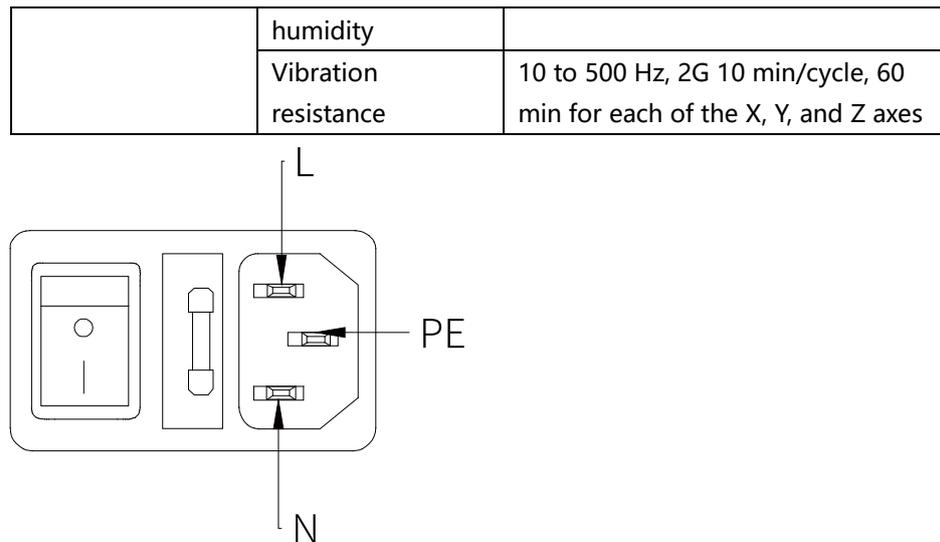
Figure 32. Power input interface
