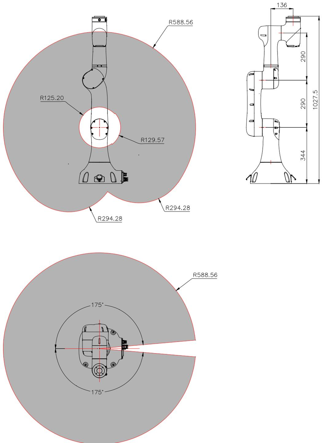
Figure 8. The working space of xMate SR3
