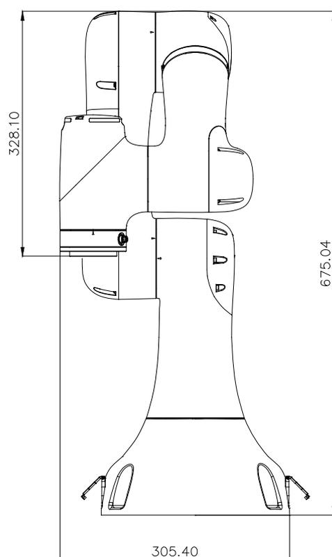
Figure 11. Reference transportation dimensions of the robot
