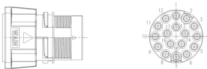
Figure 17. Handheld emergency stop and enabling device interface
