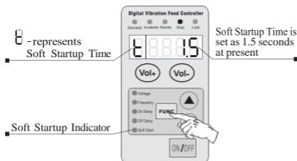
Adjustable Soft Startup Time ranges from 0.1 seconds to 9.9 seconds.
