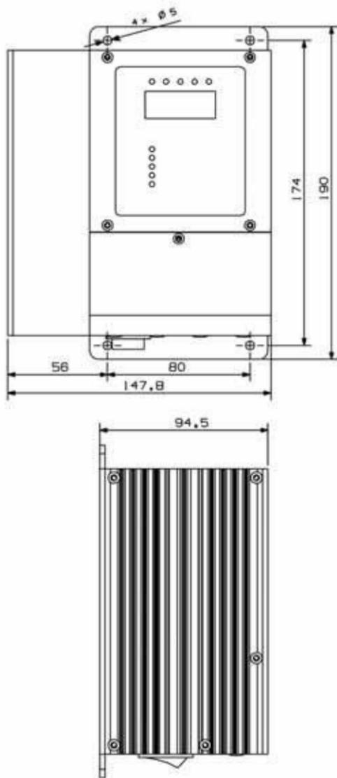
Outline Dimensions of the controller model: SDVC31-XXL and SDVC31-XXXL (unit: mm)
