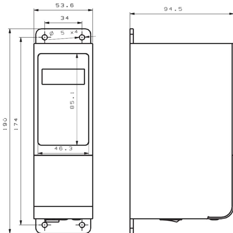
Outline Dimensions of the controller model: SDVC31-L and SDVC31-XL (unit: mm)
