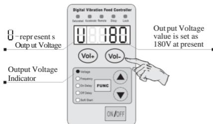
The adjustable Output Voltage of the controller series ranges from 0V to 260V
