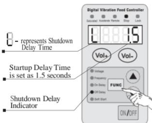
Adjustable range of the parameter is from 0.0 to 9.9 seconds
