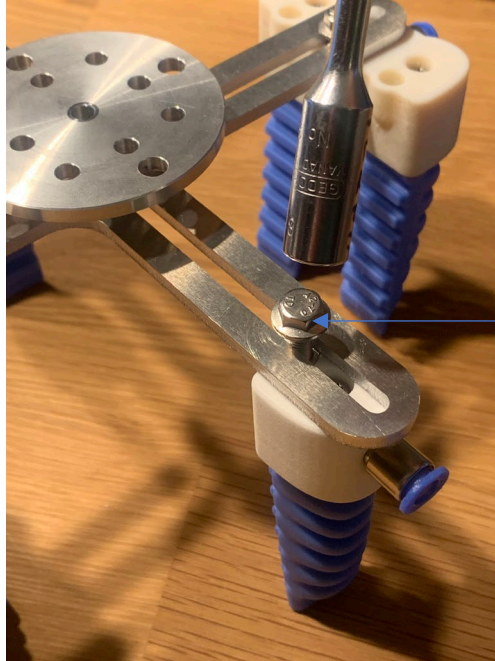
Figure 15: Mounting SoftActuator to a Plate Base
