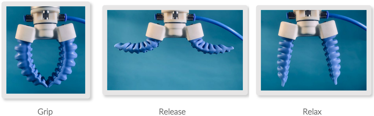
Figure 2: Three states of SoftGripping
