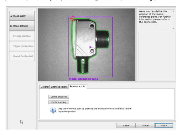
Position the reference point on the geometric centre of gravity of the model.
