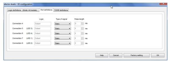
The field "Logic" shows the basic function of the pin. In the selection field "Type of signal" you set whether this is a static signal or signal pulse (pulse). In the event of a signal pulse, you can define the requested pulse length from 50...1000 ms in the following input field.
