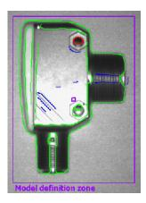
In the standard selection mode only one contour element can be selected. When you click on another element, the selected element is deselected again. A click on a free space in the image field cancels the selection made.
