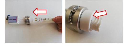
Place the module carrier onto the driver unit by positioning it flat above the interface and then sliding it down until the stop.
