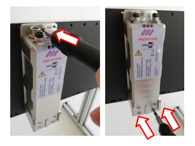
Insert the desired module into the module carrier. To do this, hold it from the outside in the front area as shown in the picture without touching the piezo element. With the sticker pointing upwards, the module can simply be inserted into the module carrier. Make sure that the module is inserted as far into the carrier as shown in the picture.
