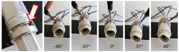
Due to its design, the piezo element does not have a circularly symmetrical crosssection. The discharge shape results in optimum angles for activation results that are as homogeneous as possible.
