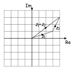
Here  $z_1 = 3 + i$  and  $z_2 = 1 + 2i$ . You can see from the diagram that  $z_1 + z_2 = 4 + 3i$ , as you would expect from adding  $z_1$  and  $z_2$  together.
