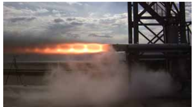
Figure 2: Static tests of the 15.2cm (6-inch) hybrid chamber
