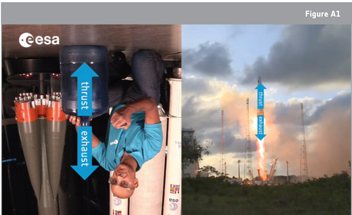
↑ To launch a rocket in space there needs to be enough thrust. This is the Whoosh bottle Classroom Demonstration Video that you can find on ESA's Education website.
