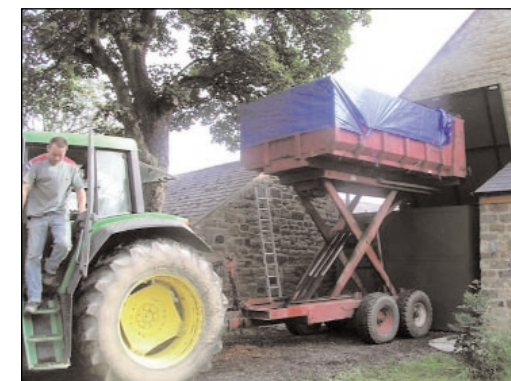
High-tipping trailer delivery
