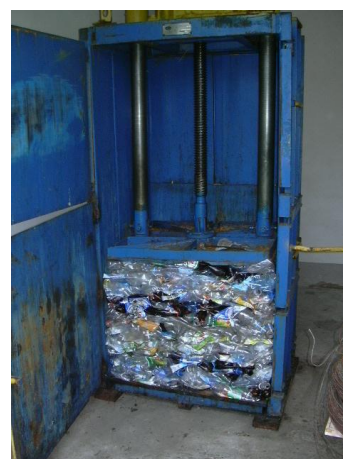
Photo 3: Simple baler for PET bottles as used in Belarus (Sophie van den Berg)
