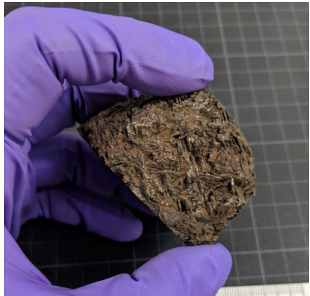
Weathered Widmanstätten pattern of meteorite Richa BM 1996M55, at the Natural History Museum of London
