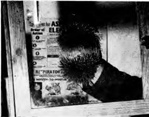
Fig. 3. The glass sheet is sandwiched vertically between the magnet and the filings; the demonstrator is holding the magnet only
