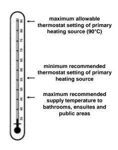
If this storage tank is installed as part of a solar water heater to an in-series continuous flow gas booster, then this requirement of AS 3498 can be satisfied provided the booster is energised, its preset outlet temperature setting is 70°C or higher and a remote temperature controller is not used.
