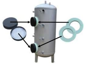
Fit the two green foam insulation rings around the upper and lower flange. Fit the two black plastic flange covers over the foam rings.
