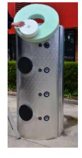
There are two round pieces of insulation that fit on top of the tank. The smaller white high density foam piece fits over the top fitting and the larger green piece fits around the white piece.
